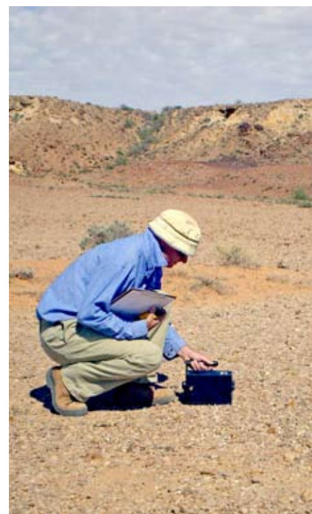
Figure 3 Validating radiometric anomalies by taking hand held scintillometer readings at Area A.
