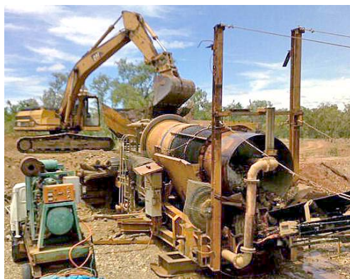
ERO gold trommel wash plant showing alluvial gravels from excavator to conveyors, November 2010.
