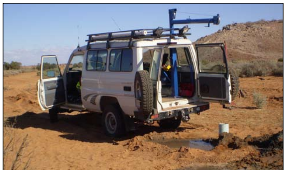
Downhole logging vehicle at Marree Project.
