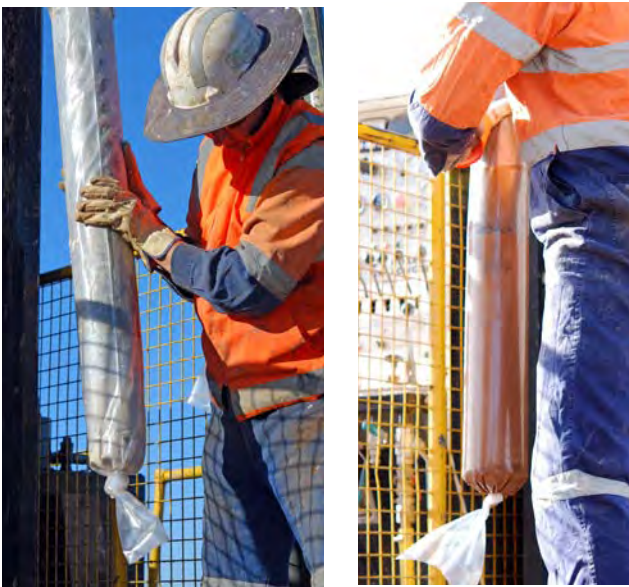
(Left) 1 m core recovery, and (Right) taking a core sample saturated with groundwater; from drillhole WT2, Wertaloona Project, South Australia, May 2011.
